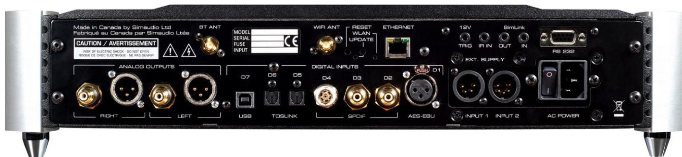
Figure 2: 680D Rear panel
