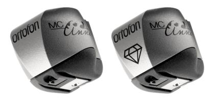
One of the important design components is Ortofon's Wide Range Damping system (WRD), in which a small, heavy platinum disc is sandwiched between two rubber absorbers, both with different properties. This ensures not only an exceptional tracking performance, but also creates a perfect damping through the entire frequency range. Because of this, distortion and resonance are virtually eliminated.
